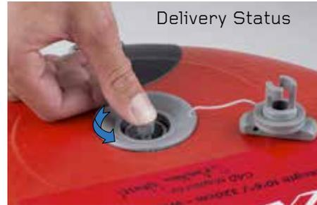
Make sure that the valve on the Fanatic Fly Air is in the outer position. The valve must be released for inflation. To release the valve, push lightly downwards and twist to the left or right (see picture). The valve is now in the upper position.
